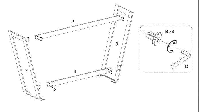
Attach part (4,5) to part (2,3) using bolt (B) with hex key (D).
