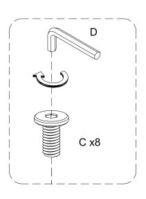
Attach part (2,3) to part (1) using bolt (C) with hex key (D).
