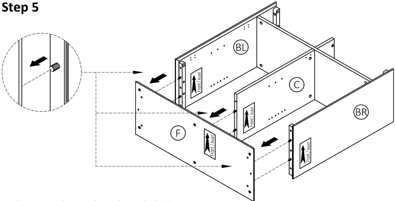
1. Align Wood Dowels with guide holes and attach Sides (BL), (BR) and (C) to Bottom Shelf (F).
