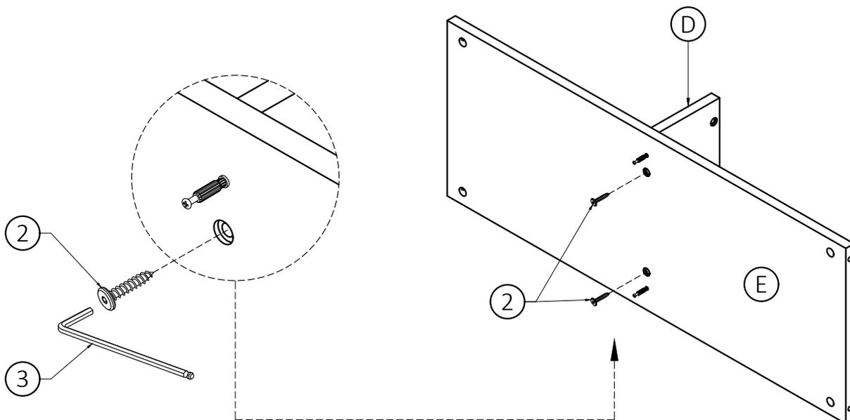
2. Use two Allen Key Screws **2** to attach Divider **D** through guide holes from Top Shelf **E** to pre-drilled holes of Divider **D**.
