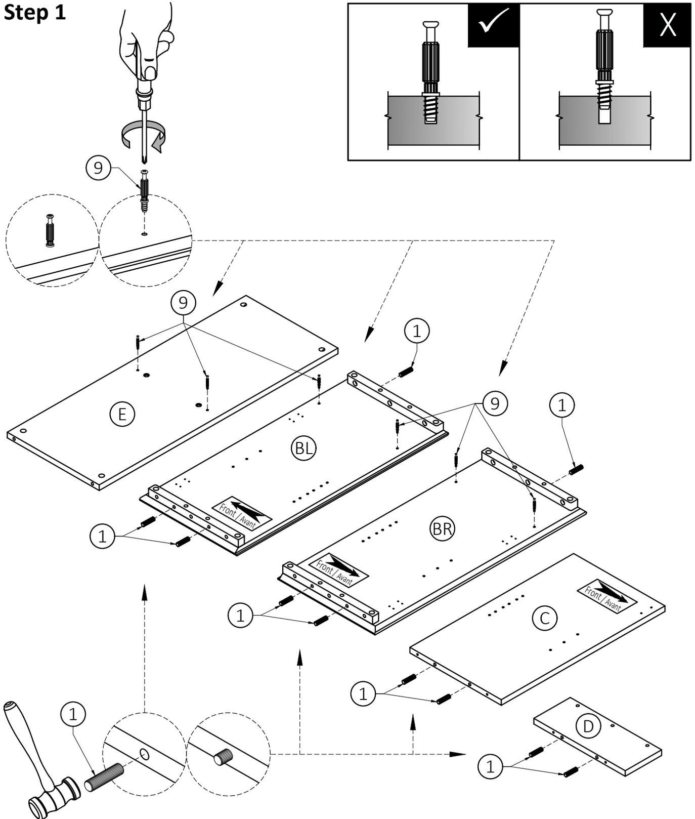
1. Attach two Cam Lock Pins ⑨ into pre-drilled holes at each Side (BL, BR) and Top Shelf (E).
