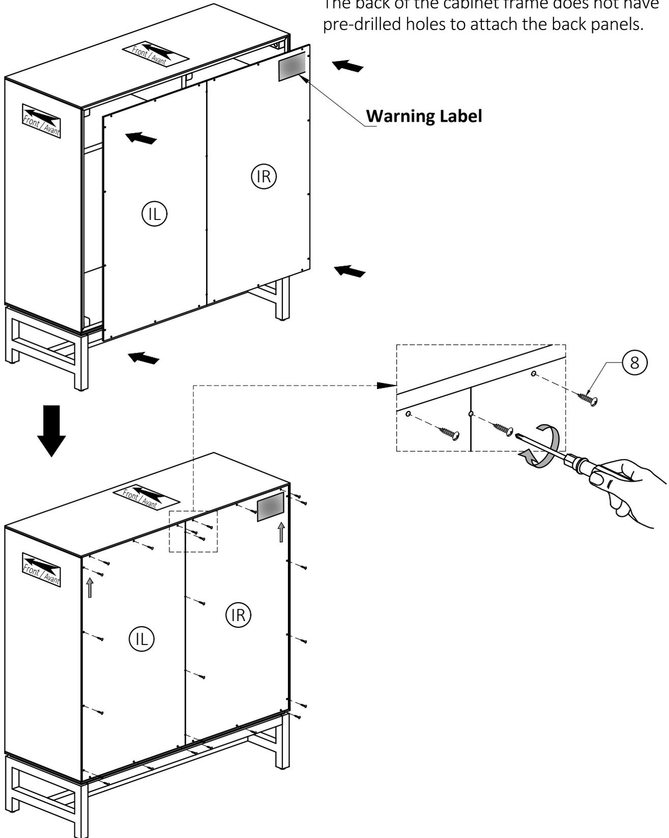
1. Attach the Back Panels (IL, IR) to back frame using Phillips Screws Round Head (8) through guide holes from Back Panels.
