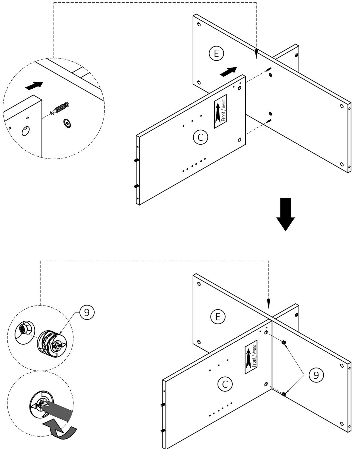
1. Align Cam Lock Pins with guide holes on Divider (C) and attach Divider (C) to Top Shelf (E).
