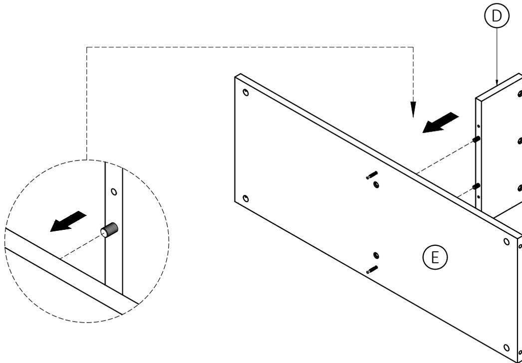
1. Align Wood Dowels with guide holes and attach Divider **D** to Top Shelf **E**.
