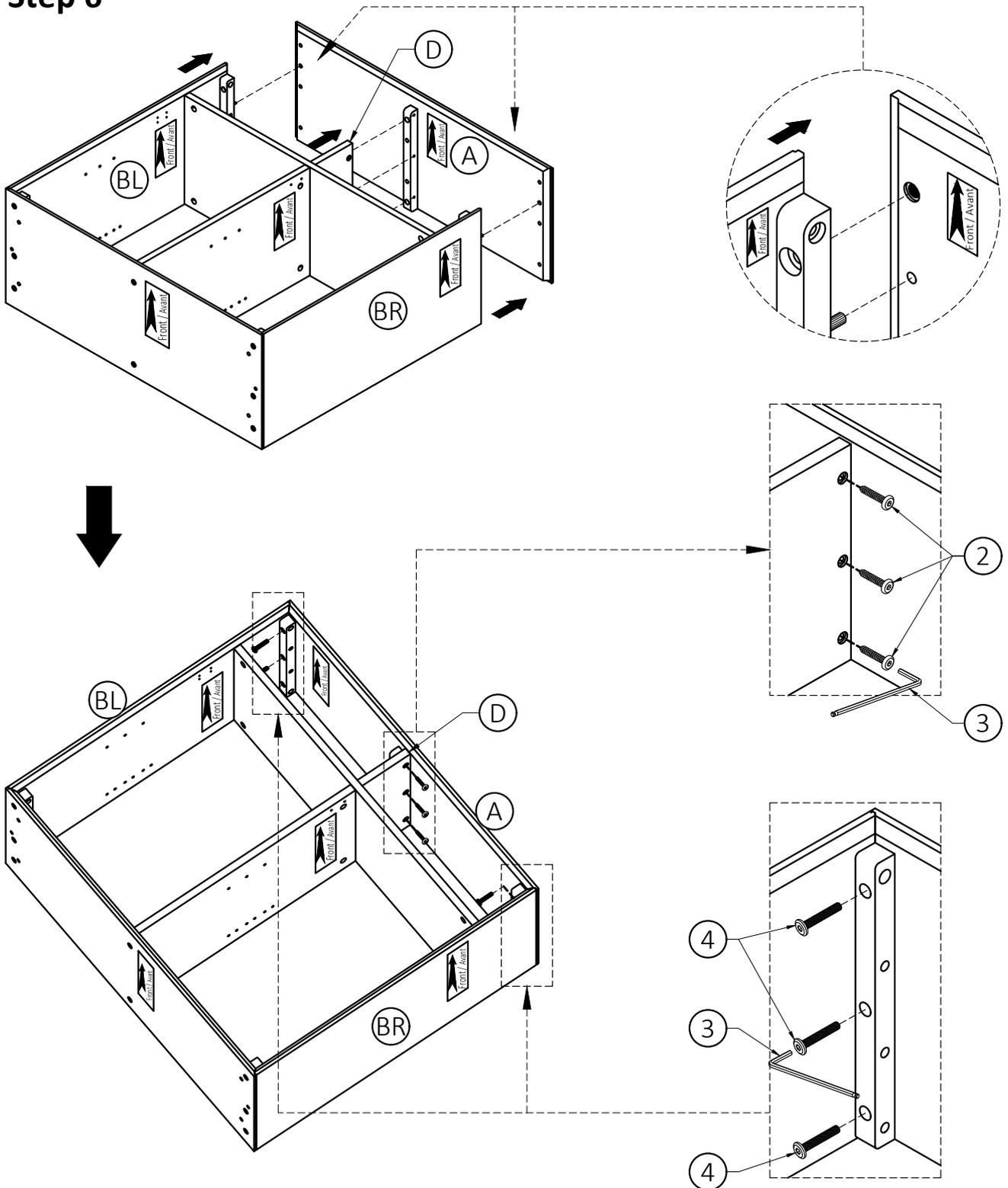
1. Align Wood Dowels with guide holes on Top (A) and attach Sides (BL), (BR) to Top (A).
