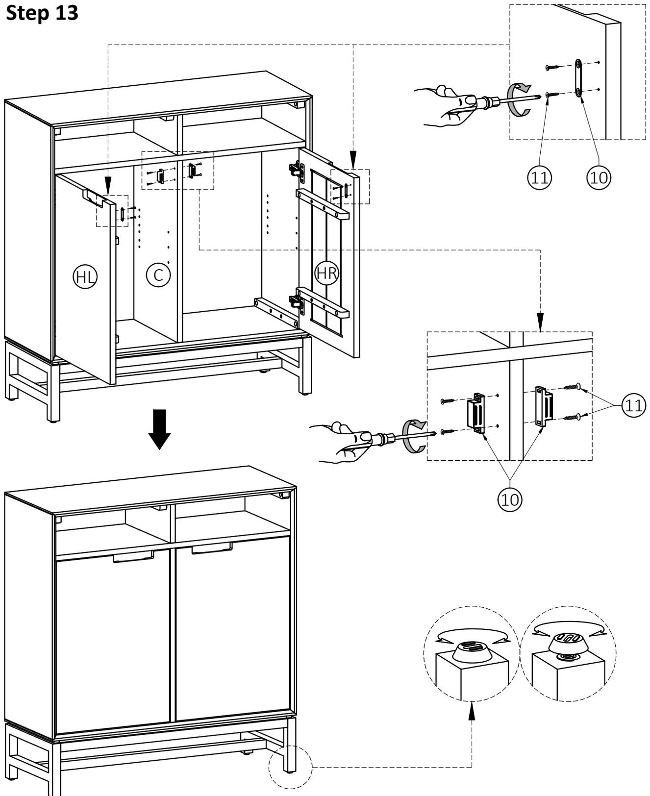
1. Attach Magnet Plates (10) to top corner of Doors (HL), (HR) using Phillips Screws (11) into pre-drilled holes on Doors (HL), (HR).
