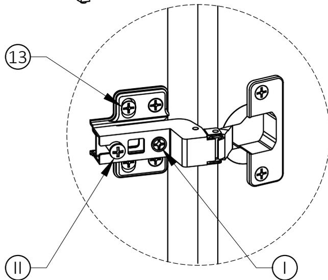
Tighten the Screw marked ⑪ to fasten hinge. The door may need to be adjusted so that all the spaces between the door and the unit sides are equal.
