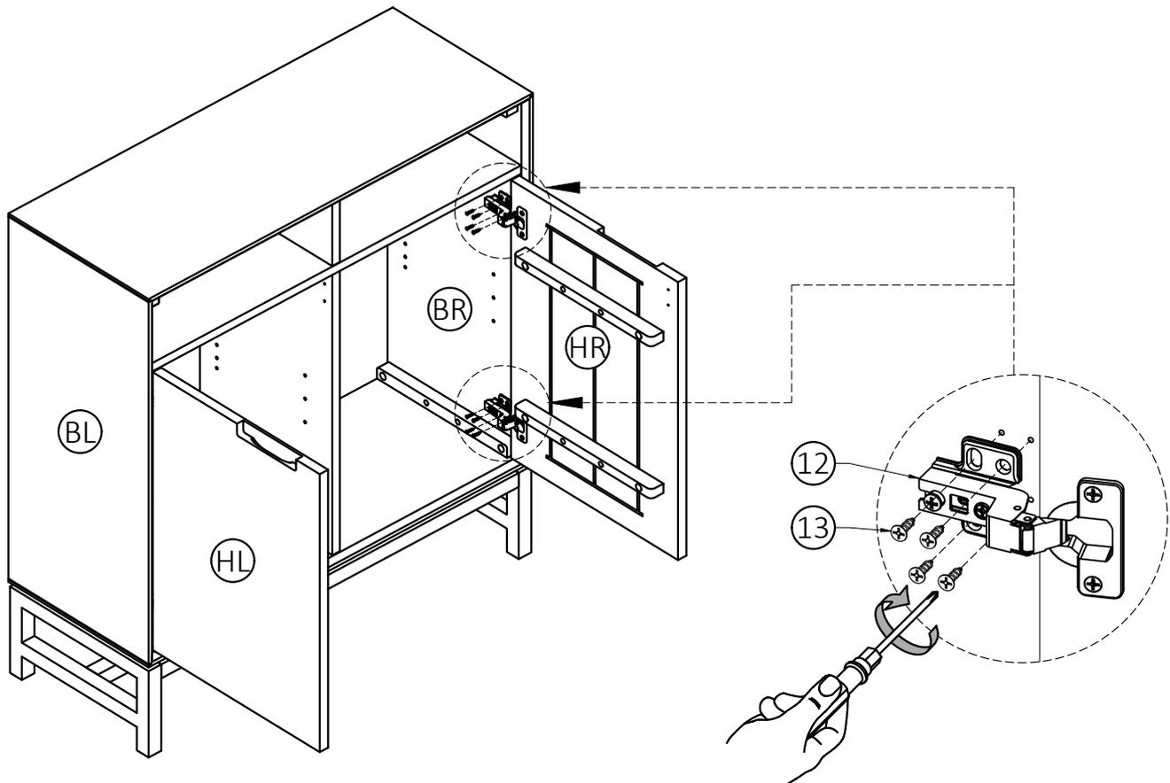
2. Attach Adjustable Hinges (12) on Doors (HL), (HR) to Sides (BL), (BR) using Phillips Screws (13) into pre-drilled holes on Sides (BL), (BR).
