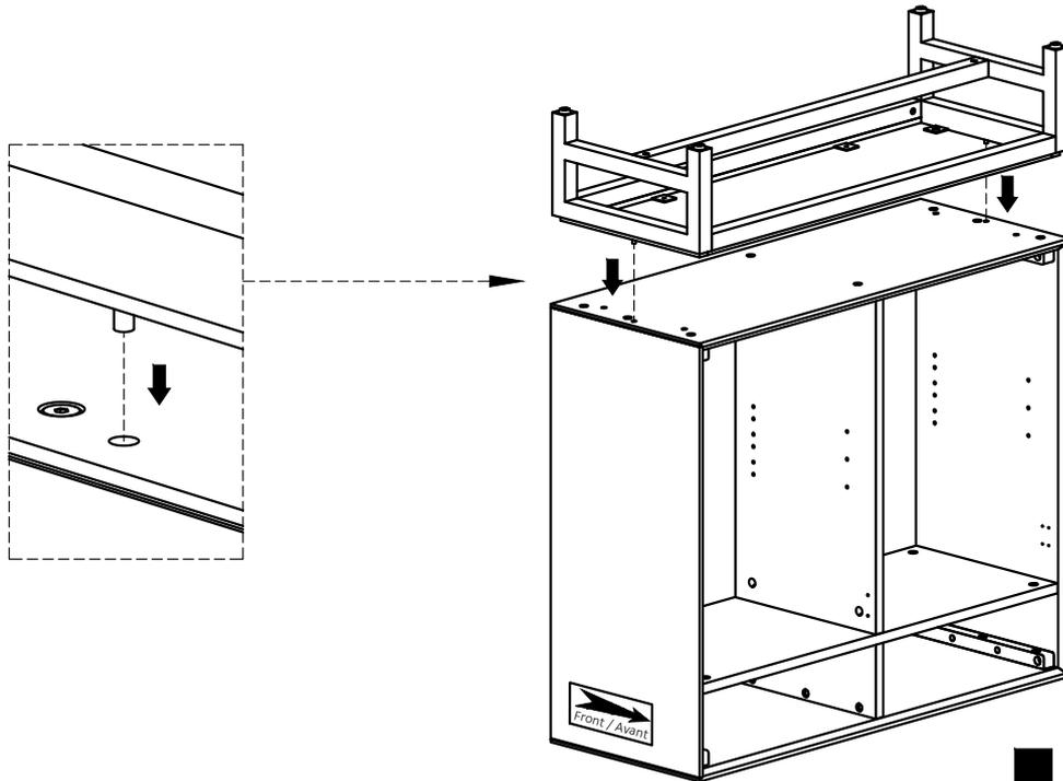
1. Align iron dowels with guide holes on wooden frame and attach the assembled metal frame to bottom wooden frame.
