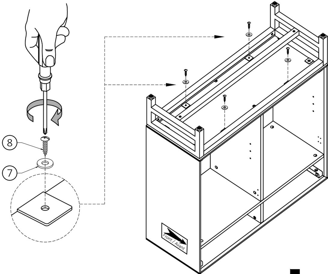
1. Use four Phillips Screws Round Head (8) and four Washers (7) to secure wooden frame and metal frame.
