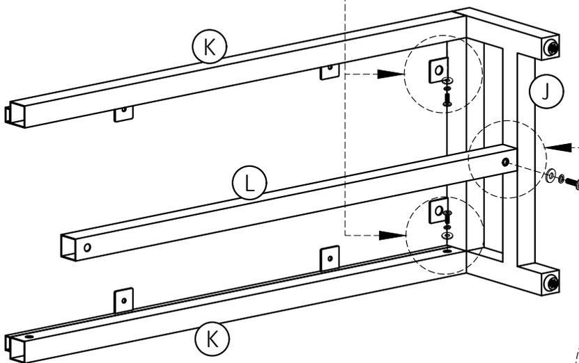
2. Use one Bolt (5), one Lock Washer (6) and one Washer (7) to secure each part (K), (L) with (J).
