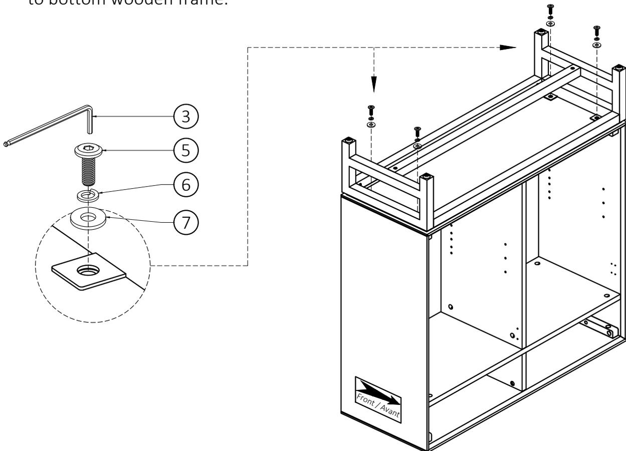
2. Use four Bolts (5), four Lock Washers (6) and four Washers (7) to secure metal frame and wooden frame .
