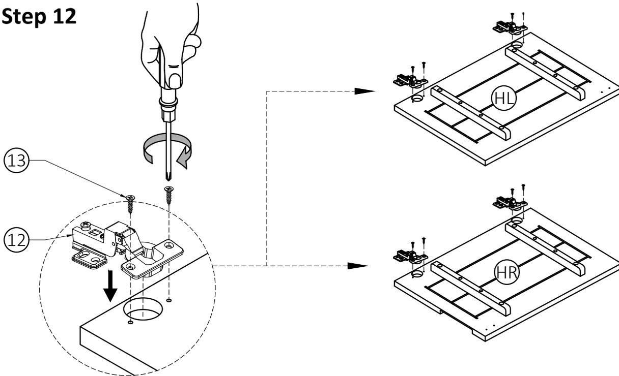
1. Attach Adjustable Hinges (12) to Doors (HL), (HR) using Phillips Screws (13) into pre-drilled holes on Doors (HL), (HR).
