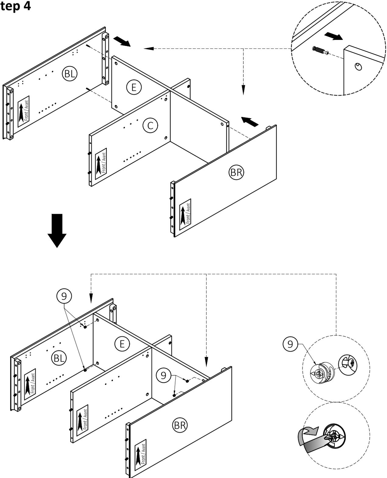
1. Align Cam Lock Pins with guide holes on Top Shelf (E) and attach Sides (BL), (BR) to Top Shelf (E).
