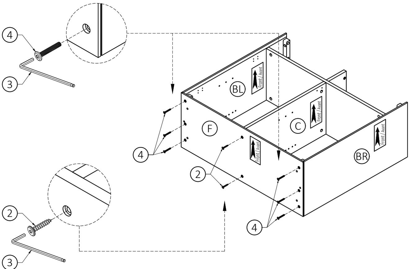
2. Use three Allen Key Bolts (4) to attach each Side (BL), (BR) through guide holes.
