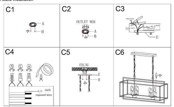
Step C1 » Unscrew knob balls (H) from canopy (E) then remove mounting plate (C).
