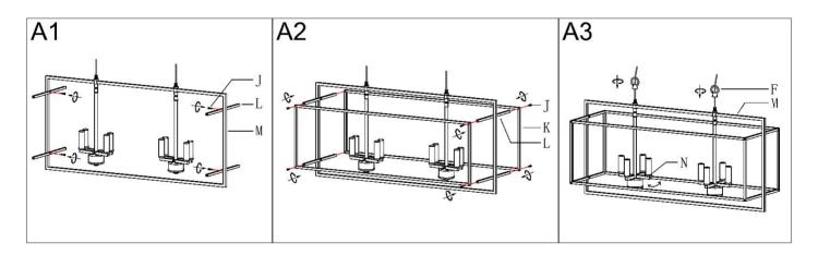
Step A1 » Fix iron tubes (L) onto outer iron square frame (M) with screws (J).
