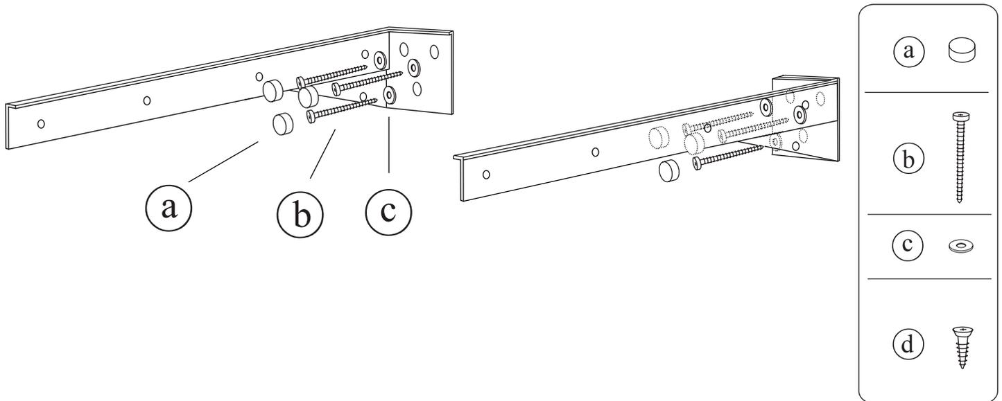
**Step 2 :** Attach the cabinet to the wall bracket.
