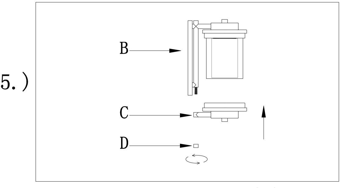
Step.5:Install the bottom cover(C) to fixture(B), using the finial(D).
