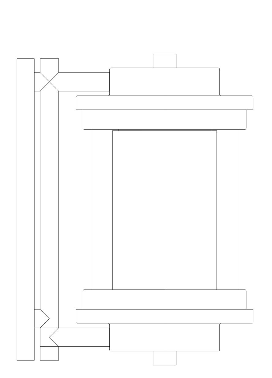
To prevent water intrusion, caulk around back-plate where fixture meets the wall using outdoor silicone sealant. Leave a small gap at the bottom to allow moisture to exit.
