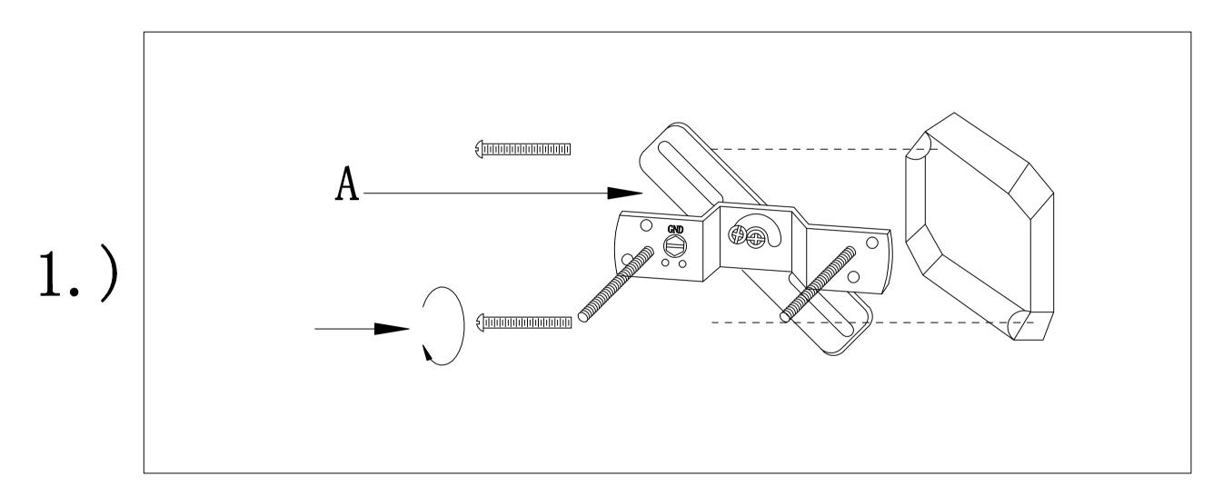
Step.1: Remove mounting bracket from fixture(B) and install to electrical box. then wire fixture to wires in outlet box. Copper wire is for Ground.
