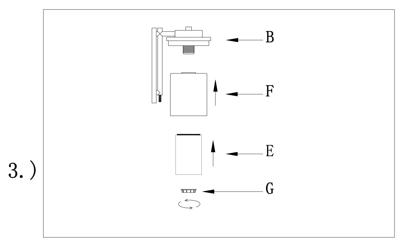
Step.3:Install the outside glass(F) and the inside glass(E) to fixture(B), using the screw ring(G).
