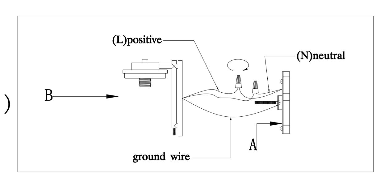
Step.2: Attach back plate to mounting bracket and tighten ball nuts so fixture meets wall. Caulk fixture where back plate meets the wall with silicone sealant.
