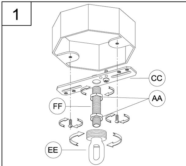
1. Install the chain holder (EE) onto the nipple (FF). Next, loosely thread the hex nuts (AA) onto the nipple (FF) and then thread this assembly onto the mounting strap (CC). Install this assembly to the outlet box using the mounting screws supplied with the outlet box (not included).
