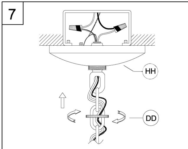
7. Tuck the wires into the junction box and slip the canopy (HH) over the chain holder. Thread the screw collar (DD) onto the chain holder to secure the canopy tightly to the ceiling.
