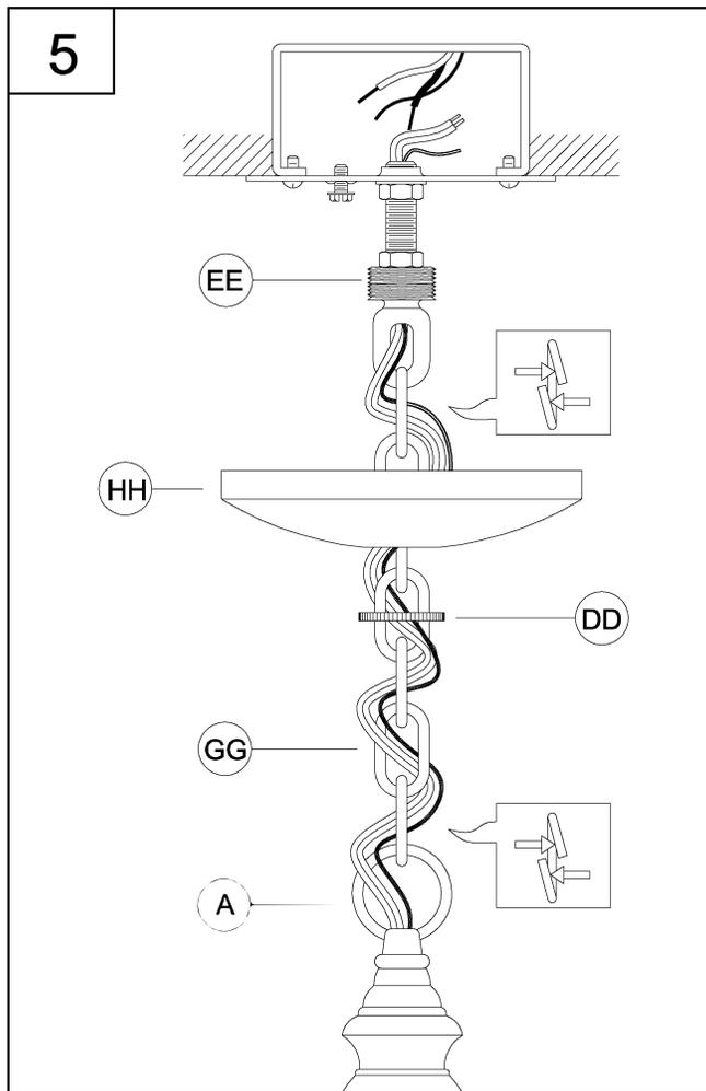
**NOTE:** During this step, determine the hanging length of your fixture by removing chain links (GG) and optionally cutting the electrical and ground wire to length.
