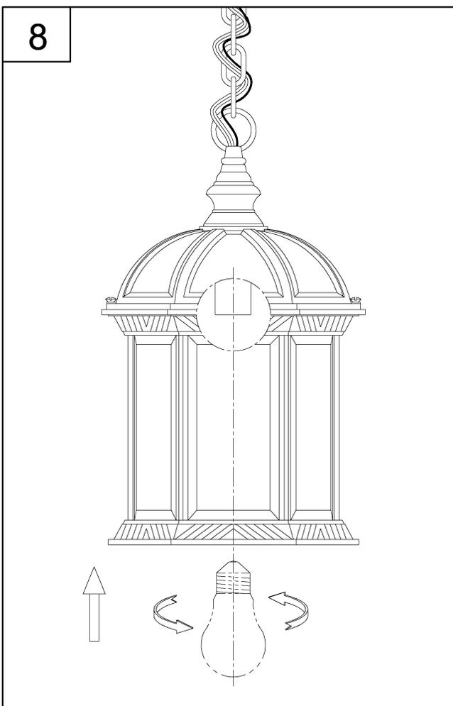
8. Thread the lamps (not included) into the fixture sockets. Use 60-watt MAX incandescent medium base, SBCFL or SBLED.
