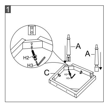
Step 1: Assemble legs (A) with seat frame (C). Use L-wrench (H3) to lock with 4\*bolts (H2).
