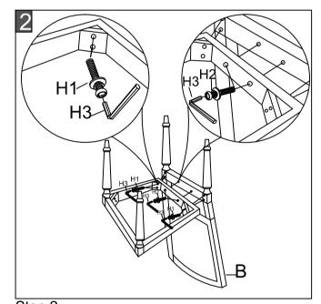
Step 2: Attach chair back (B) with the assembled seat frame/legs. Lock with 6 bolts (2\*H2 & 4\*H1) by using L-wrench (H3).
