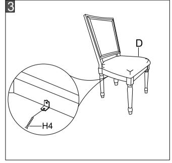
Step 3: Place seat cushion (D) on top of seat frame. Lock with angle irons & screws (H4).Assembly is completed.
