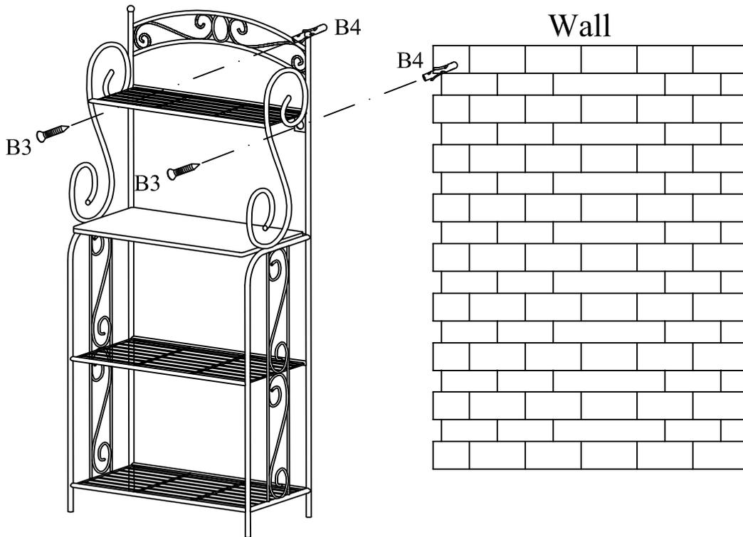
For your safety, please attach this unit to the wall by Screws B3 and Anchors B4.
