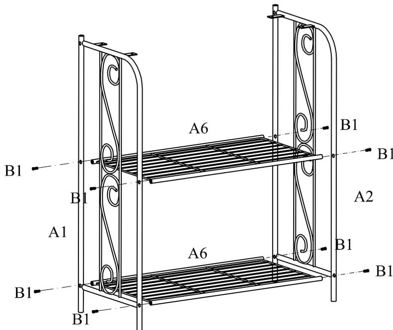
Assemble Lower Side Frames A1&A2 to Lower Net Racks A6 using Bolts B1.
