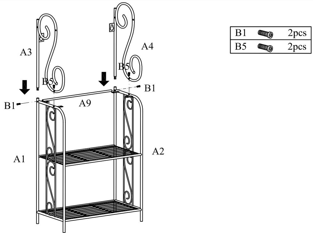
1).Insert Upper Side Frames A3&A4 to Lower Side Frames A1&A2 as shown above.
