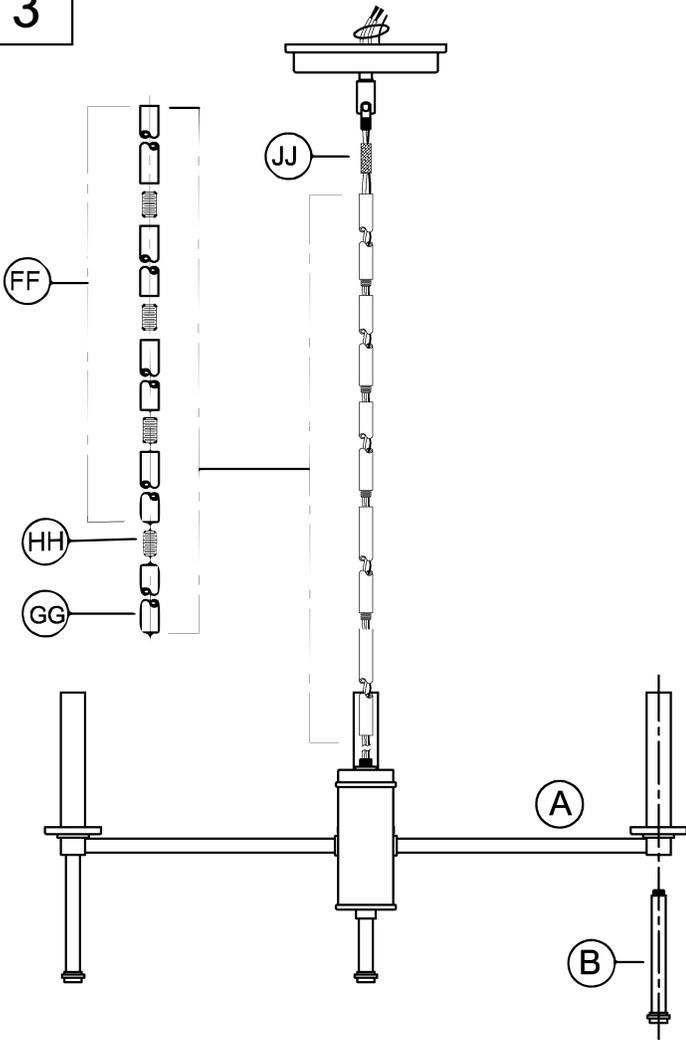
NOTE: During this step, determine the hanging length of your fixture by adding or removing stems. The electrical and ground wire may also optionally be cut to length.
