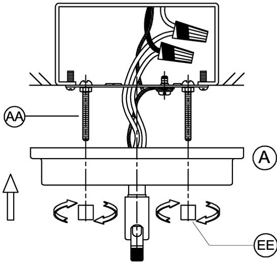
5. Pass the screws through the two holes in the canopy. Secure the fixture (A) to the screws (AA) using the two cylinder nuts (EE). Tighten securely.
