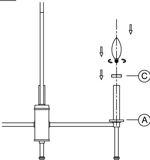
6. Attach the small cup (C) to the glass holder of fixture (A).
