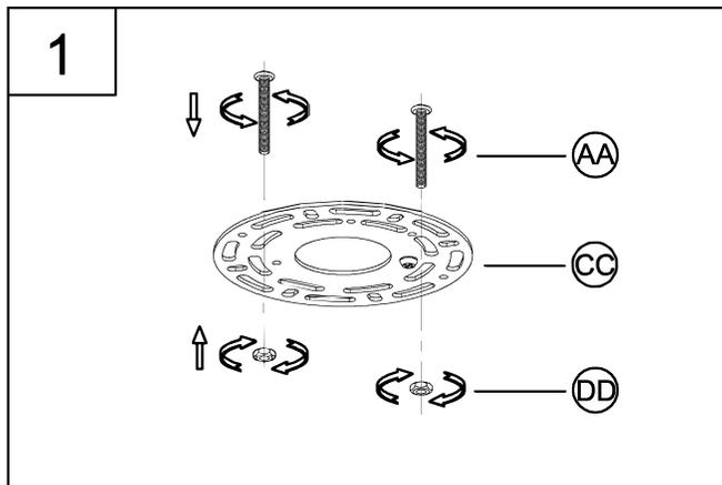
1. Loosely thread the screws (AA) and the hex nuts (DD) onto the round mounting plate (CC) as shown. You now need to adjust the screw length according to the fixture canopy depth.
