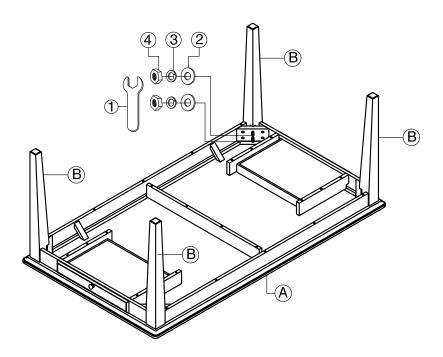
Place the Table Top (A) up side down on the floor with a piece of cloth or carpet underneath to prevent the finish from scratching. Attach the Leg (B) to the corner of Table Top (A) and secure with Flat Washer (2), Lock Washer (3) and Hex Nut (4). Fully tighten with Wrench (1). Repeat this step for the remaining three legs. Product assembly is now completed.
