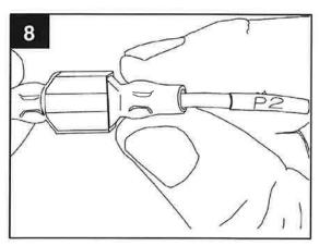
9. Insert the blower link (male plug) into the power link (female port).
