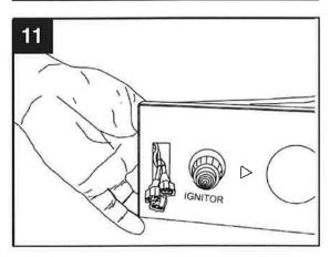
12. Connect AUTO, OFF, MAN wires to the three corresponding male ports on the Rocker Switch (E). Match the "Auto" wire to the symbol "—" and the "Man" wire to the symbol "—" on the rocker switch (E).
