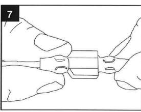
8. Insert the female plug (marked with P2) into the corresponding male port, which is on the black power supply wire (marked with P2).
