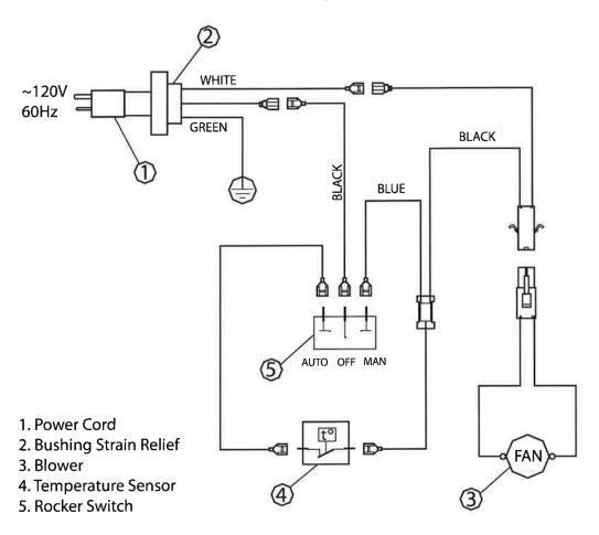
**NOTE:** If any of the original wire as supplied with the appliance must be replaced, it must be replaced with a wire of at least an equal temperature rating.
