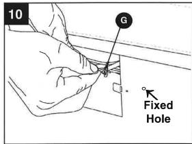
11. Insert AUTO, OFF, MAN wires through the Rocker Switch opening.
