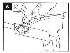
7. Insert the female plug on the white power supply wire (marked with P1), into the corresponding male port (marked with P1).
