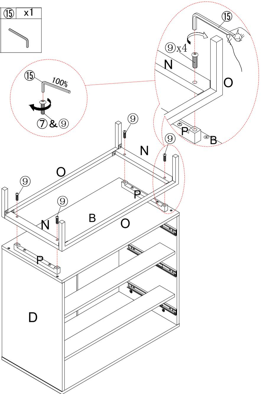
**STEP12: Use bolt ⑨ to attach the preassemble leg(O)&(N) to the corresponding hole of part(P), tighten bolt ⑨ with allen key ⑮.**
