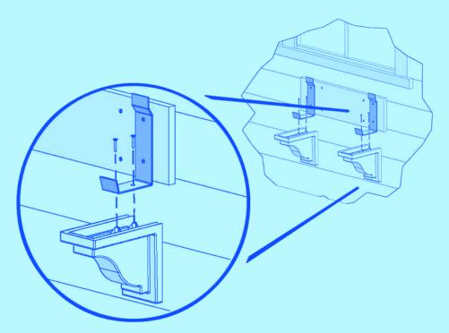
Secure each decorative bracket to the bottom of the wall mount brackets using two 3/4 inch screws. The decorative brackets are sold in pairs so we recommend installing them on the outside brackets. The molded brackets are only decorative so there is no need to over tighten the screws.
