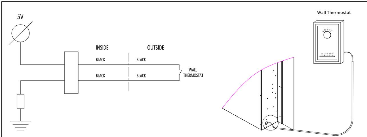
**NOTE:** The wall thermostat will be functioning when the heater is on the TEMP. setting.
