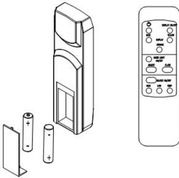
For remote to function make sure the heater is plugged in and the main power switch located on the bottom left hand side is at position I.
