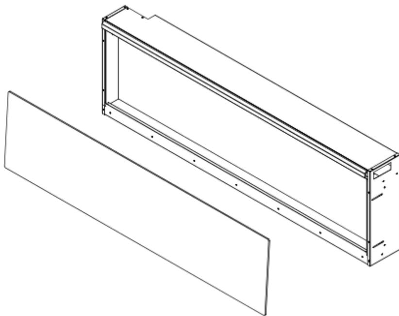
3. Unscrew the 2 screws located on each side and take off the inner side steel panels.
