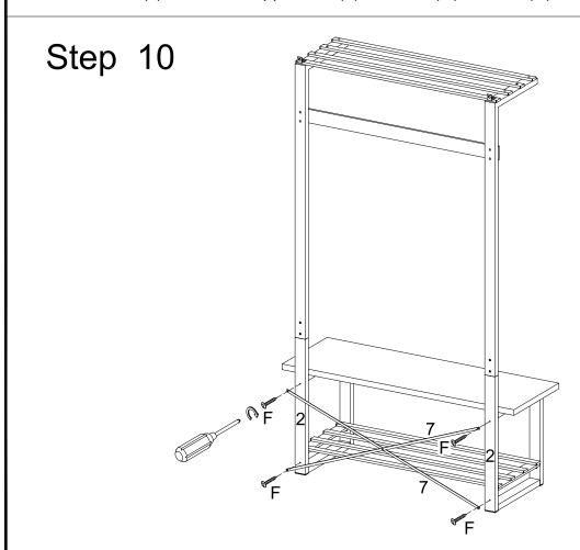
Secure support bar (7) to side frame (2) with screw (F).
