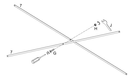
Use wrench (J) to secure support bar (7) with bolt (G) and nut (H).
