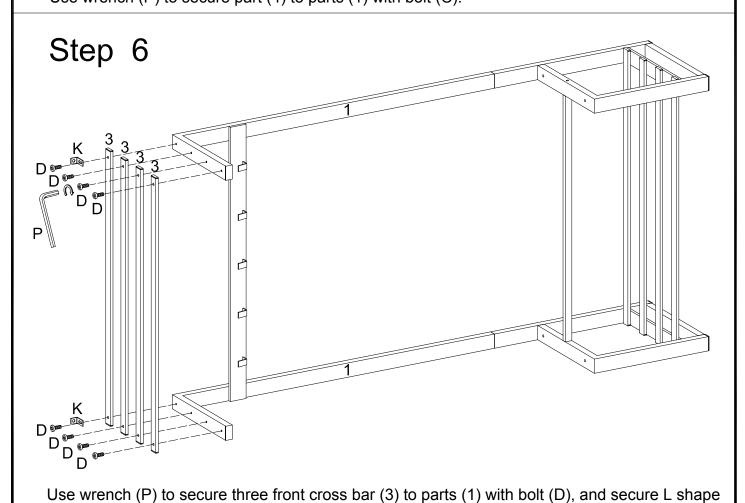
bracket (K) and bolt (D) to last cross bar(3) to parts (1).
