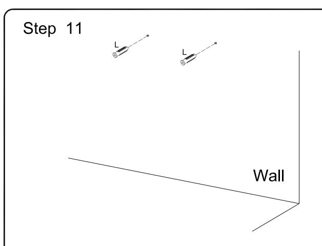
Place unit in desired location and mark the wall for anchor location. Insert plug (L) into wall as per diagram.
