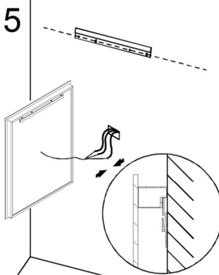
Hang the mirror to the wall and make sure the bracket in the back of the mirror lineup with the mounting bracket properly.
