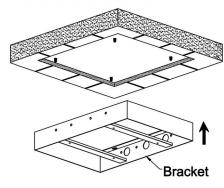
6. Install the washer and spring washer with explosive screw heads, and then use a copper sleeve wrench to lock the nut to the bracket, and the bracket is flush with the ceiling.
