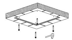
4. Use a socket wrench to remove the lock nut, spring washer, and flat washer counterclockwise.
