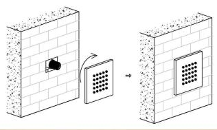
3. Use a hexagonal wrench to rotate clockwise to install the 1/2 threaded joint on the wall side spray joint. (Note: The 1/2 threaded joint has an internal threaded end facing outward).
