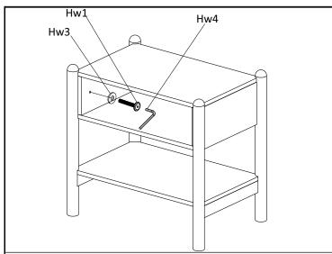
STEP4 Use the Allen Key (HW3) to screw in the Allen Bolts (HW1) with the Flat Washers (HW2) as shown.
