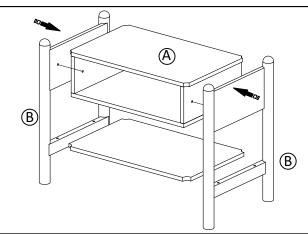
STEP2 Place the Bedside (A) upside down on a clean ,soft surface. Align the screw holes on the legs (B) with the screw holes on the top(A).
