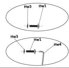
STEP3 Put the Flat Washer (HW2) on the Allen Bolt (Hw1) as shown.
