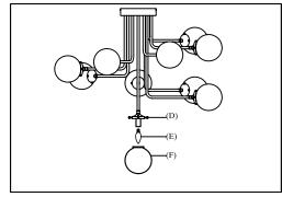
step3: Loosen the lock screws (D). Install E12 bub(E) and attach glass (F). Secure glass (F) by tightening lock screws (D).
