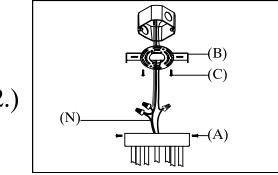
step2: Wire fixture to wires in outlet box. Copper wire in canopy is for grounding. Install fixture to mounting bracket(B) using screws (A) on the sides to secure.
