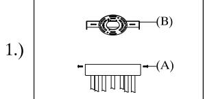
step1: Remove mounting bracket (B) from fixture and install to electrical box. Mark where screws at ends of bracket meet the ceiling. Remove mounting bracket from ceiling. Drill holes using 3/16"  $\pm$  drill bit where marked. Install mounting bracket to outlet box and attach anchors to secure bracket at ends.
