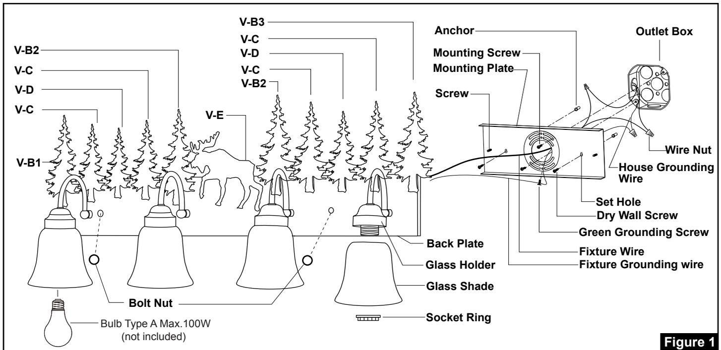
1. Unscrew two bolt nuts, and remove the mounting plate from the back plate.
