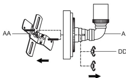
2. Attach cross bar (AA) to outlet box (not included) using outlet box screws (BB).
