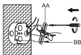
3. Strip 3/4 in. of insulation from fixture wire ends. Twist stripped ends together with pliers (not included), black to black (power), white to white (neutral). Snip ends. Wrap the ground wire from the outlet box around the green screw preassembled on the cross bar (AA), and then connect the ground wire from the outlet box to the ground wire from the fixture.
