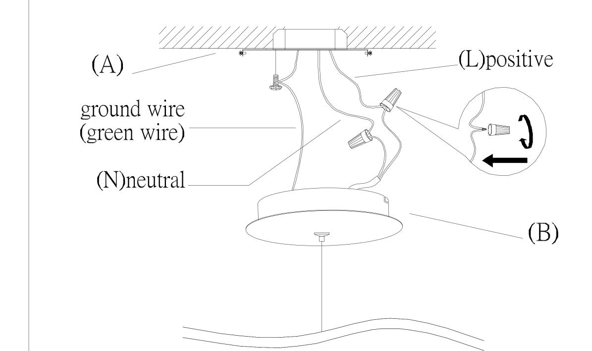
Step 2: Use push pins to adjust wires to desired mounting height. Wire fixture to wires in outlet box. See dual plastic wire instructions for more details. Install Green wire to Ground Screw.
