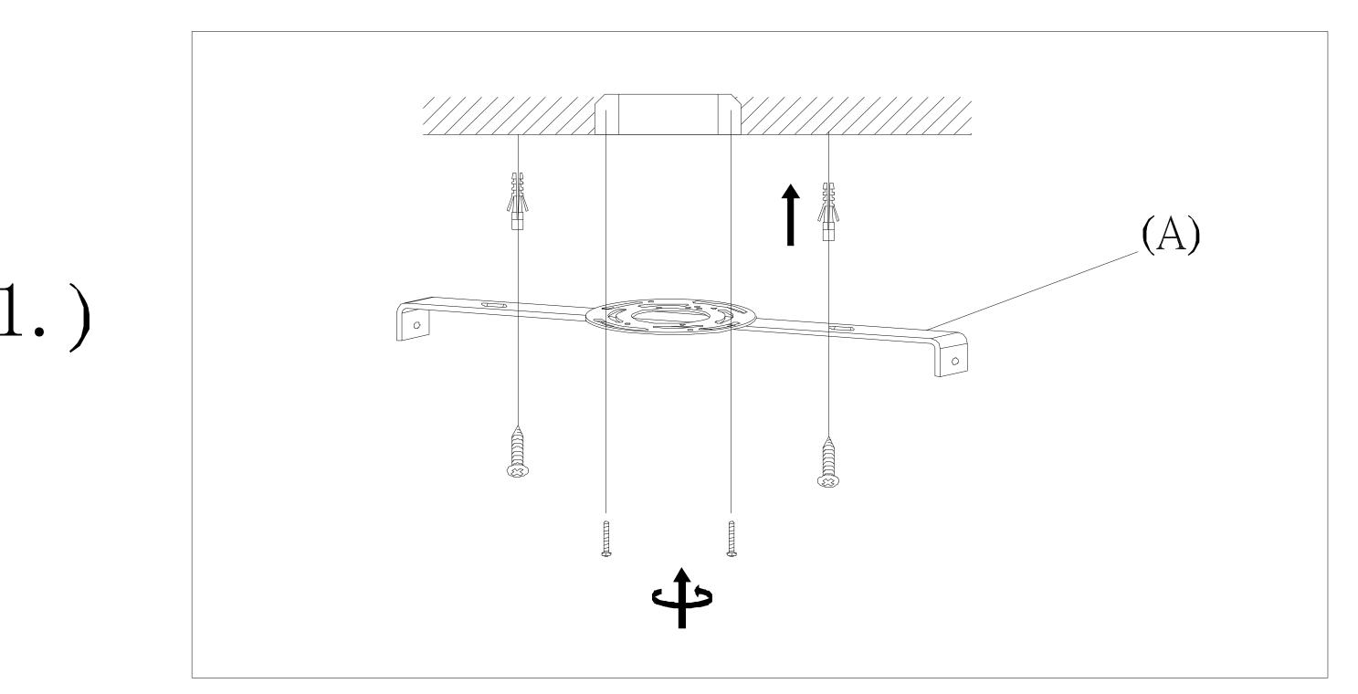
Step 1:Remove mounting bracket from fixture and install to electrical box Mark where screws at ends of bracket meet the ceiling. Remove mounting bracket from ceiling. Drill holes using 3/16"± drill bit where marked. Install mounting bracket to outlet box and attach anchors to secure bracket at ends.
