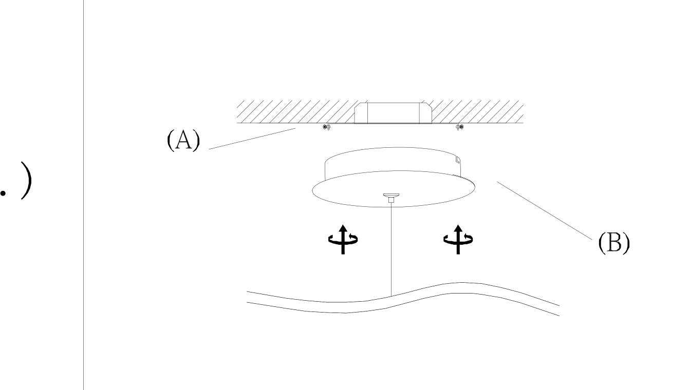
Step 3: Install Body (B) to Mounting Bracket (A) and tighten screws on the sides of the canopy to secure
