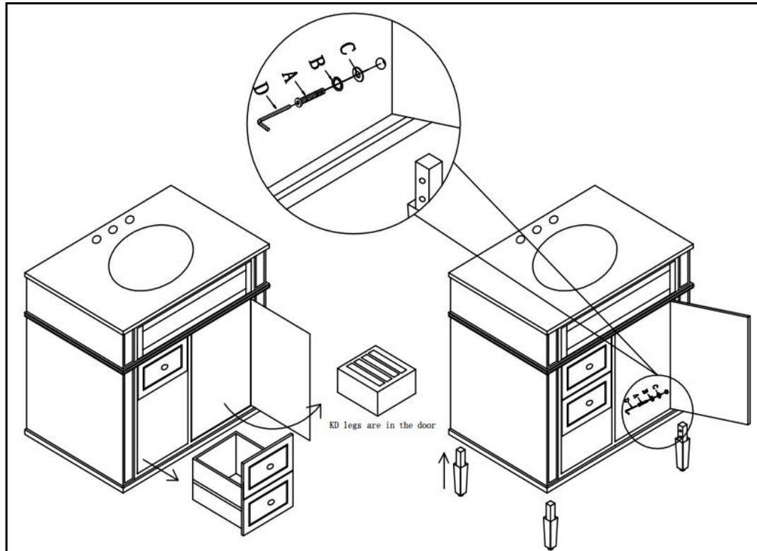
1. Take out the drawer and open the door      2. Insert foot, and mounted on the screw
