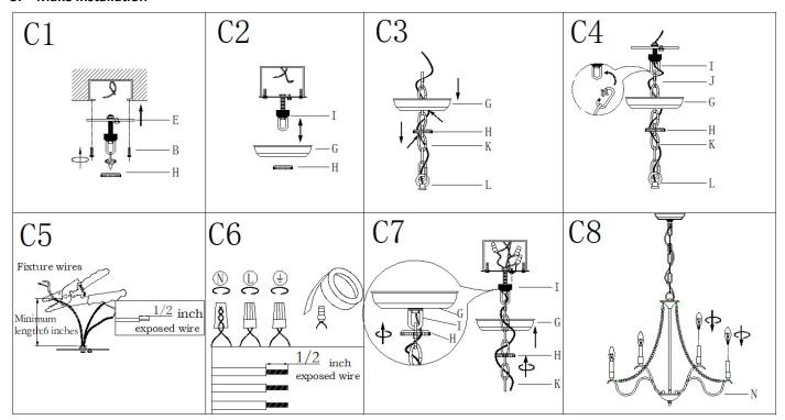
Step C1: .Attach the single bar (E) to outlet box with mounting screws (B). The side of single bar marked "GND" must face out
