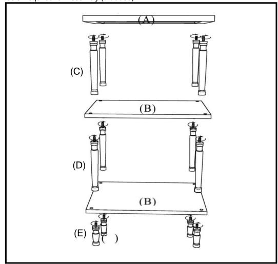
Screw all the feet (E) to the shelf (B), and then screw the legs (C) (D) to the shelf (B) and top (A)
