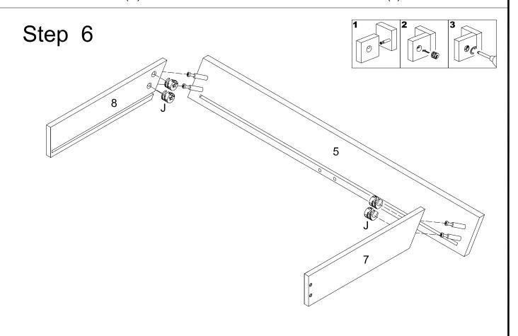
Attach the Front Panel and secure it with the Cam lock (J) for both side.
