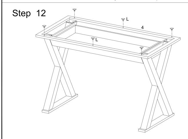
Insert the Rubber Suction Cups (L) into the per drilled hold on the Frame (4).
