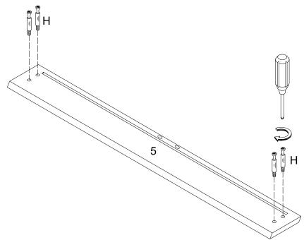
Insert the Cam Bolt (H) with the Screw Driver to the Drawer Front Panel (5).
