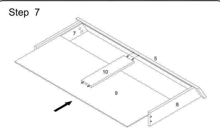
Attach support bar (10) to the drawer front panel (5) with wooden dowels. Upside Down the Drawer unit and Slot in the Drawer bottom board (9) to the unit.
