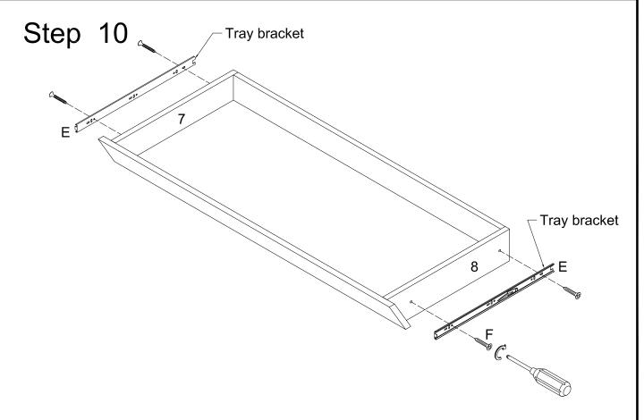
Attacher the tray bracket of keyboard tray sliders (E) on the Drawer Side Panels (7) & (8) by using Screws (F) and the Screw Driver.
