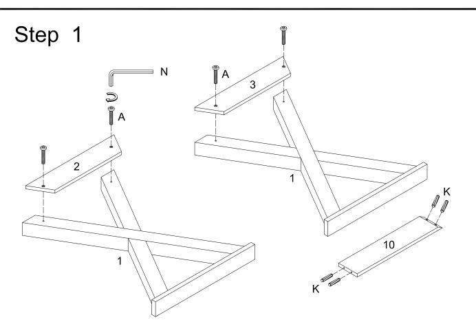
Attach Side Panel (2) & (3) with Screws (A) to the Legs (1), Insert the Wooden Dowels (K) into the Support Bar (10).
