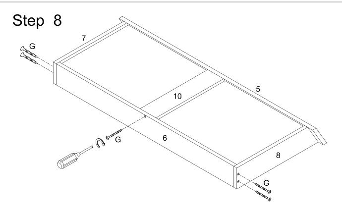
Attach the Side Panels (7) & (8), Support Bar (10) to the Drawer Back Panel (6) and secure it with the Screw (G).
