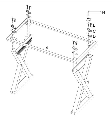
Right up both Legs (1) and place the Frame (4) on top and secure it by using Bolts (B), Spring washers (C), Washers (D) and the Wrench (N).
