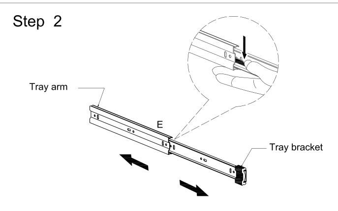
Disassemble keyboard tray slider (E) by sliding the tray arm and the tray bracket apart. Depress the small lever on the tray bracket and carefully pull the two pieces apart. Repeat this process for both keyboard tray sliders (E).
