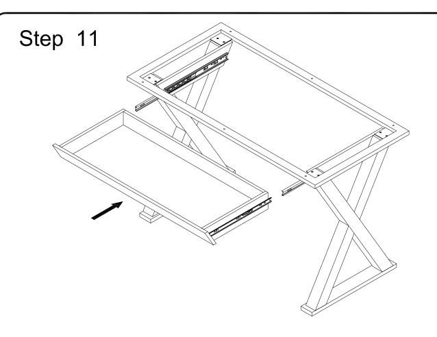
Insert the Drawer Rails to the Frame Rails carefully for the drawer setup.
