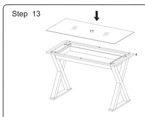
Place the Tempered Glass (11) on top of the Frame (4) and finidhed.
