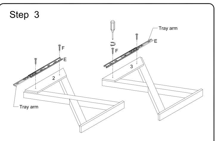
Attach the tray arms of keyboard tray sliders (E) on the Panels (2) & (3) and secure it by Screws (F).
