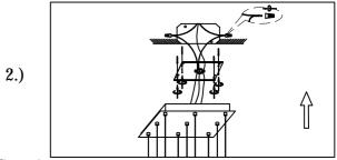
Step.2: Wire fixture to wires in outlet box. Green wire is for Ground.
