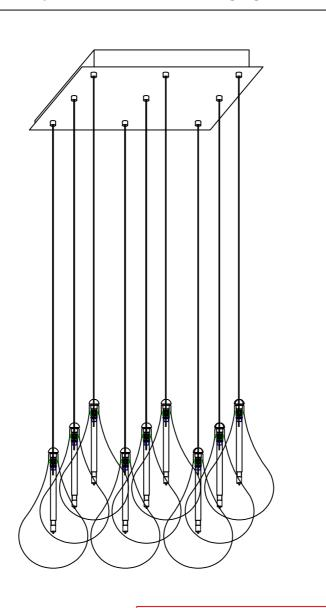
WARNING: Wires need to be connected to driver found in canopy and should not be connected directly to power source or a short may occur
