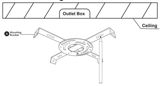
Raise mounting bracket (A) to the ceiling. Mark location for the plastic anchors (B). Use drill to drill holes for plastic anchors (B). Insert plastic anchors (B) into hole.
