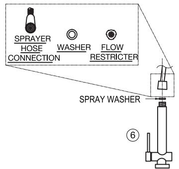
6. Attach sprayer to the female connection of sprayer hose by hand and tighten until secure.
