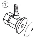
2. Remove metal nut, rubber ring, and metal ring from the faucet. Attach metal-braided hoses to the faucet.
