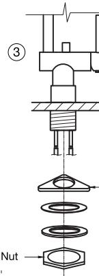
4. If the spray holder is not attached, attach the spray holder and spray hose to the faucet and tighten the screw until the spray holder is secure.
