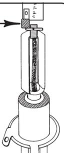
**22 ALTERNATELY** install two different arms into washer. Line up holes in arms with dimple in washer. Use lock washer and nut to secure arms in place.
