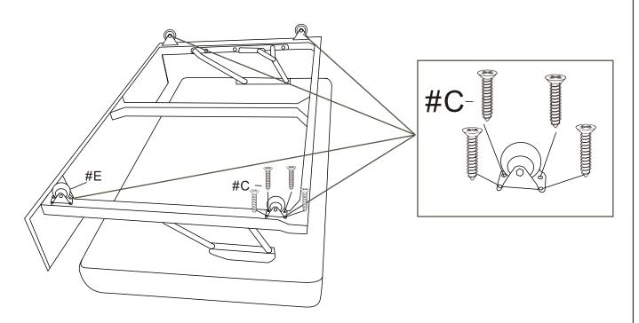
Assemble the wheels onto the sleeper
