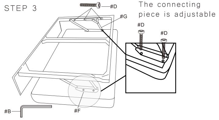
Assemble the left and right mechanisms to the sleeper cushion
