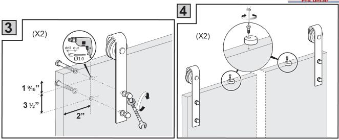
Drill out holes in the door using a 10mm routing drill bit as pictured. The bottom of the doors should be routed at this time in order to accept the floor guide.
