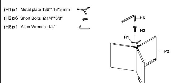
Step 3. Attach the assembled support panels (P2) to the bottom of table top (P1) as shown below.
