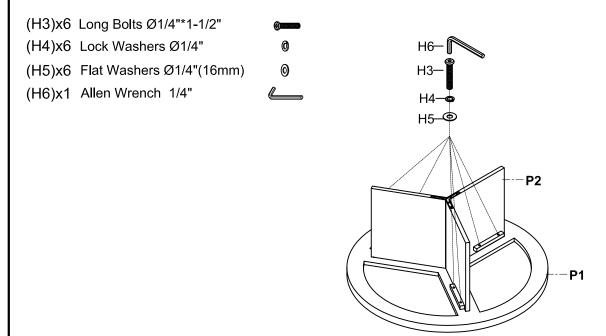
Step 4. Securely tighten all bolts with Allen wrench(H6), turn the assembled table to an upright position, make sure the table is level, aligned properly. Assembly is complete. **Failure to follow these instructions may cause the bolts to misalign during assembly.**
