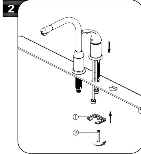
Place handle assembly through side hole in sink. Secure handle assembly with washer (1) and nut (2). Make sure that the slot on nut is facing up. Make sure handle is facing forward and it swings equally in both directions.
