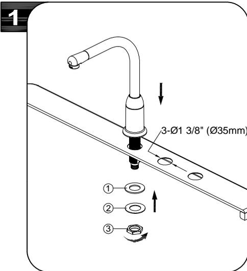
Shut off water supplies. Place spout through mounting hole in sink. Secure spout with rubber washer (1), metal washer (2) and nut (3).
