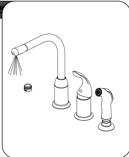
**Important:** After installation is completed, remove aerator assembly. Turn on hot and cold water supplies. Turn handle to full open position for one minute. Check for leaks. Replace aerator.
