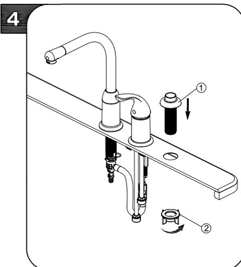
Insert hose guide (1) through the sink hole. From underneath sink, secure hose guide (1) by screwing mounting nut (2). Do not overtighten.
