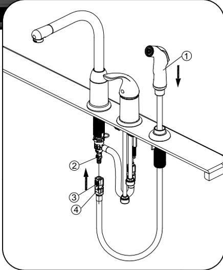
Insert side spray hose (1) through hose guide and sink. Align block (2) and tabs (3) on quick connect (4). Push quick connect housing firmly upward and snap onto receiving block. Pull down moderately to ensure connection has been made. If it is necessary to remove quick connect, squeeze tabs on hose between index finger and thumb, then pull down to disconnect.
