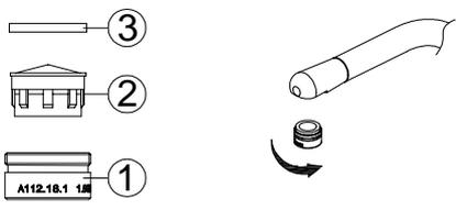
This faucet ships with a 1.5GPM aerator installed. An optional 2.2GPM aerator is also included in the box.
