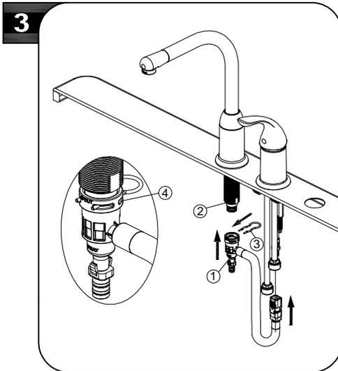
Push diverter connector (1) all the way up until completely seated onto tube (2). Slide clip (3) into diverter holes (4) to secure unit.
