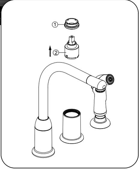
Loosen cartridge nut (1) by turning it counter-clockwise and lift out the cartridge (2). Insert new cartridge and retighten the cartridge nut. Reinstall the handle.
