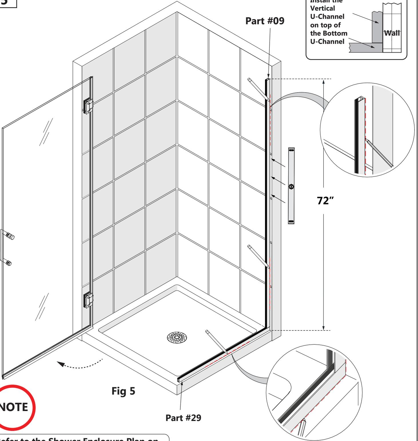
Refer to the Shower Enclosure Plan on pages 5-6 for the proper location of the U-Channels based on the model size
