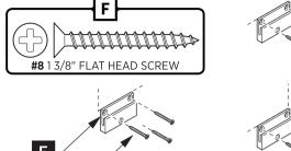
IMPORTANT: Consult an expert for the proper screws/bolts to use when attaching to various constructions. Screws provided <u>do not</u> attach to all wall construction types. Anchors are not required if brackets are installed in stud.
