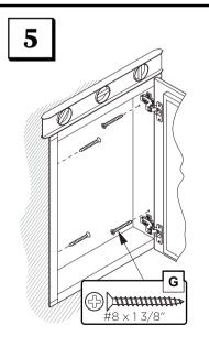
Level, then secure the medicine cabinet with the screws (G) through the mounting holes into the framing studs.
