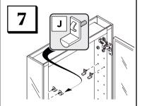
Push and twist the snapin pins (J) into place.
