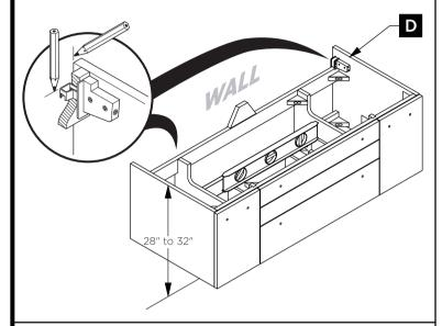
Apply a bid of silicone and hang the cabinet (D) on the brackets (E).
