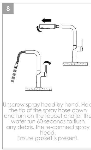
Unscrew spray head by hand. Hold the tip of the spray hose down and turn on the faucet and let the water run 60 seconds to flush any debris, then re-connect spray head.
