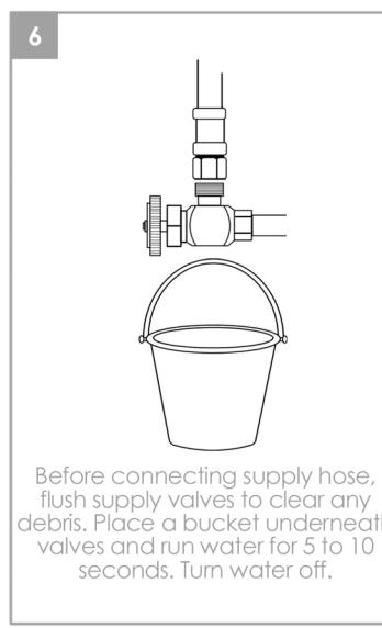
Before connecting supply hose, flush supply valves to clear any debris. Place a bucket underneath valves and run water for 5 to 10 seconds. Turn water off.
