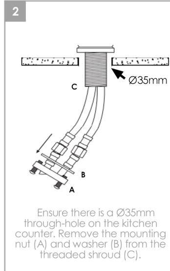
Ensure there is a Ø35mm through-hole on the kitchen counter. Remove the mounting nut (A) and washer (B) from the threaded shroud (C).
