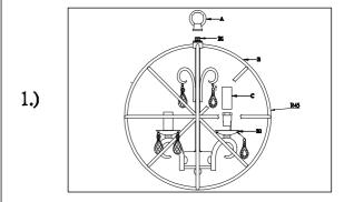
Step.2: Hang the crystal (CRP0034) on the metal cup(B2)
