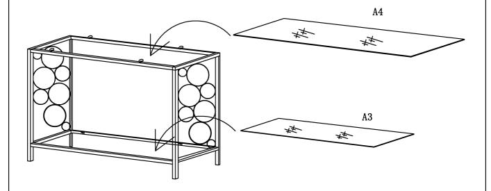
Place Glass Top A4 & Bottom Glass A3 onto the frames as shown Note: Please tighten Bolts B1 at this point.
