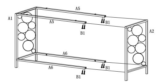
Assemble Connecting Bars A5 & A6 to Right Frame A2 using Bolts B1.
