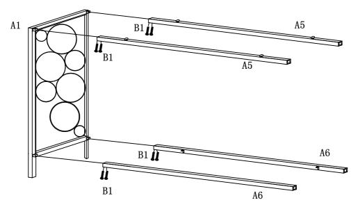
Assemble Connecting Bars A5 & A6 to Left Frame A1 using Bolts B1.
