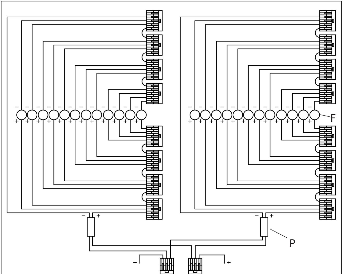
**NOTE: All positive pendent (H) contacts are wired together and all negative pendent contacts are wired together to form a parallel circuit.**
