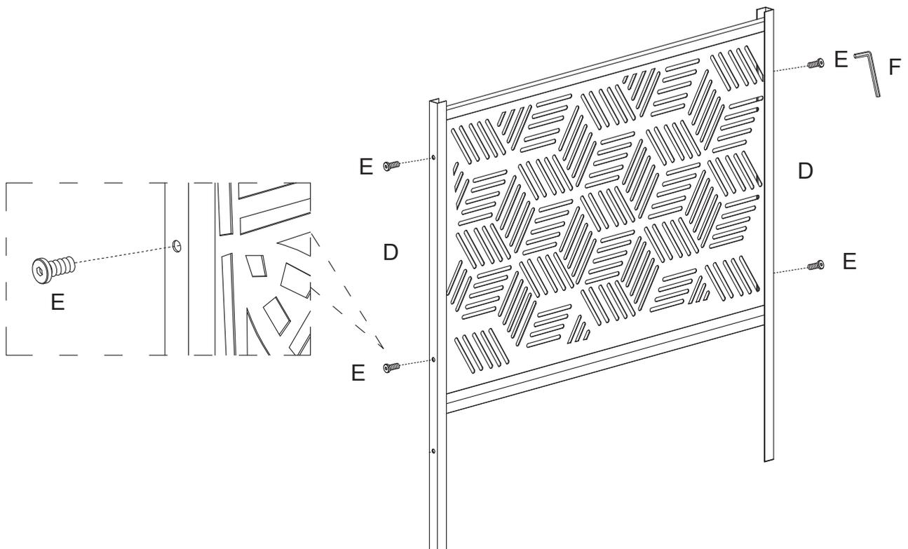
**STEP 5** Attach the assembled part 2 onto the assembled part 1. Secure the two assembled parts using the remaining 2 Bolts (E) with the Allen Key (F).
