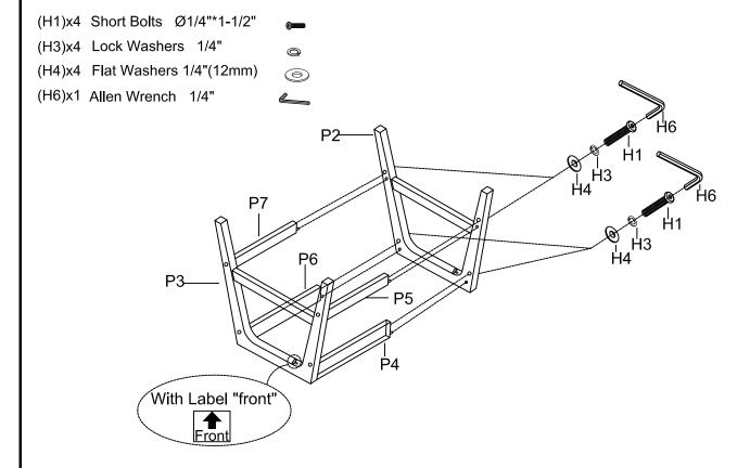
Step 3. Attach the assembled base to the bottom of the chair top (P1) as shown below. Securely tighten all bolts by Allen wrench (H6), but do not over tighten the bolts.
