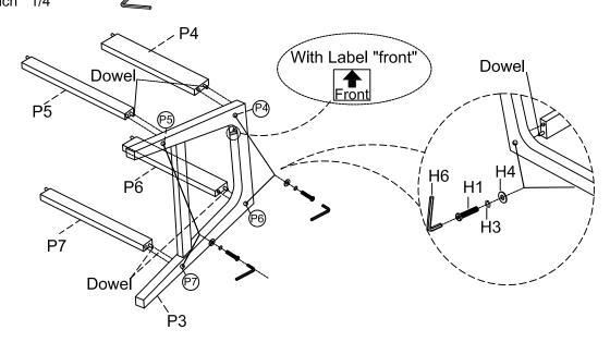
Step 2. Repeat the step 1 to attach the left leg (P2) according to the label (front) to the rails and stretchers (P4,P5,P6,P7) as shown below. Securely tighten all bolts by Allen wrench (H6), but do not over tighten the bolts.
