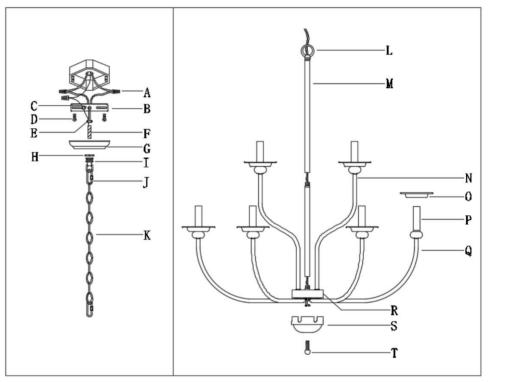
Step A1:Carefully thread stem(M) onto the top of wire house (R) until snug .
