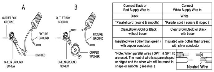
Twist plastic wire connector until wires are tightly joined together, wrap each connector with approved electrical tape. Be sure that no wire strands are exposed and carefully tuck all wires into the outlet box.
