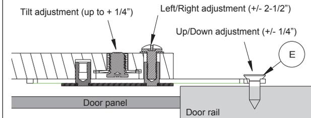
Attach the door panel and adjust as shown. (NOTE: four (4) #8 x 5/8 Flat Head Phillips Wood Screws are provided. Determine door panel rail thickness before using.)
