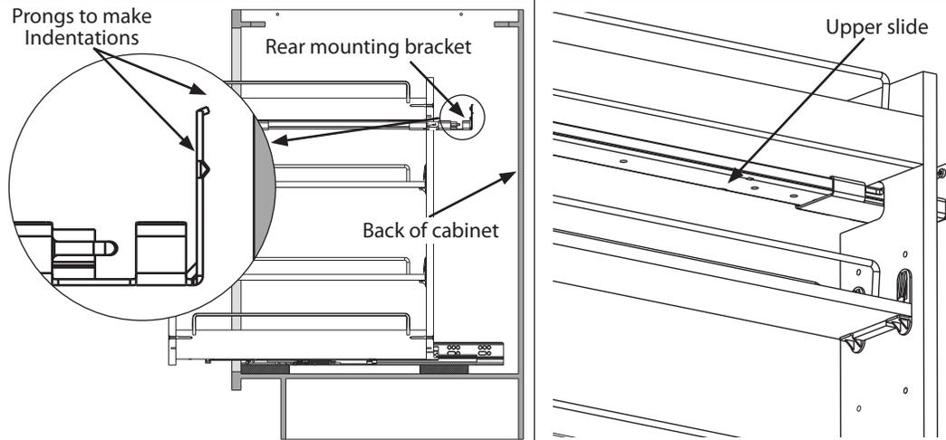
Once the unit is centered and leveled, mark the base location of the unit. With one hand holding the undermount slide, carefully pull the organizer partially open to gain access to the upper slide. Firmly grasping the upper slide, tap it against the back of the cabinet. The rear bracket should make small indentations in the back of the cabinet.
