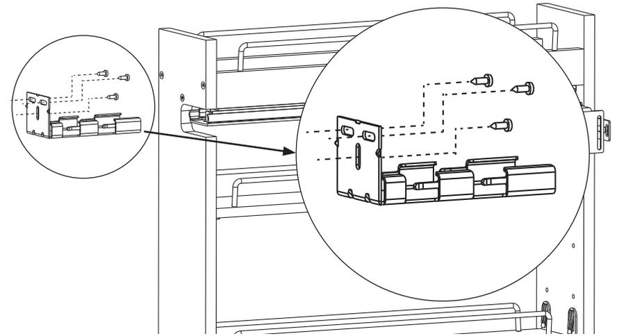
Taking the unit from the cabinet, remove the rear mounting bracket for installation. Align the rear bracket prongs with the indentation marks on the rear of the cabinet and secure with three (3) #8 x 5/8" Pan Head Wood Screws in the slots as shown.
