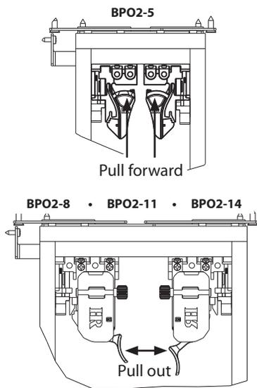
Remove the base from the unit by releasing the slide clips. Place the base back into the cabinet in the previous location. Install with the four (4) #10 x 1-1/4" Pan Head Wood Screws provided in the four pre-drilled holes in the runners.
