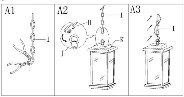
Step A1 » By measuring, determine the correct number of links needed for proper hanging height. Using the chain pliers, disconnect and discard the unwanted part.
