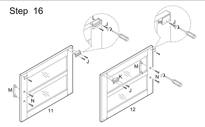
Attach handles (M) to doors (11, 12) using short bolts (N). Attach door stopper plates (H) to doors (11, 12) using screws (J). Attach door hinge (L) to door (11) using screws (J). Attach door hinge (K) to door (12) using screws (J).
