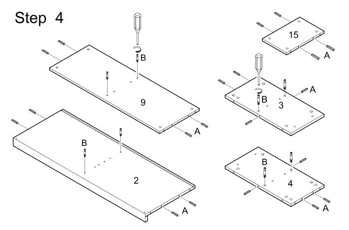
Insert dowels (A) into panels (2,3,4,15) and shelf (9). Screw cam bolts (B) into panels (2,3,4) and shelf (9).
