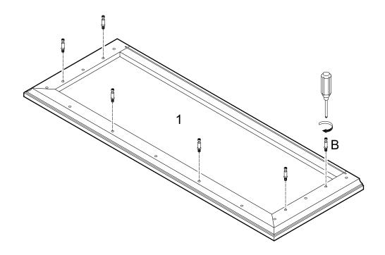
Screw cam bolts (B) into stand top (1).
