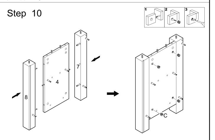
Attach legs (7,8) to panel (4) using cam bolts and dowels as guides. Insert cam locks (C) into panel (4) and tighten with a screwdriver.
