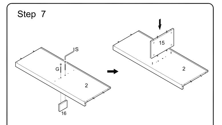
Attach support leg (16) to panel (2) using long bolts (G). Tighten long bolts (G) with wrench (S). Attach panel (15) to panel (2) using cam bolts and dowels as guides.
