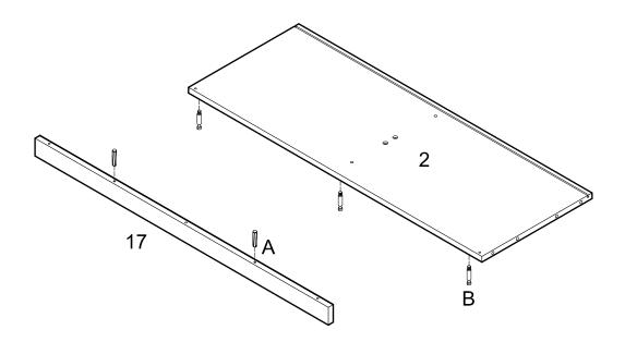
Screw cam bolts (B) into panel (2). Insert dowels (A) into slat (17).
