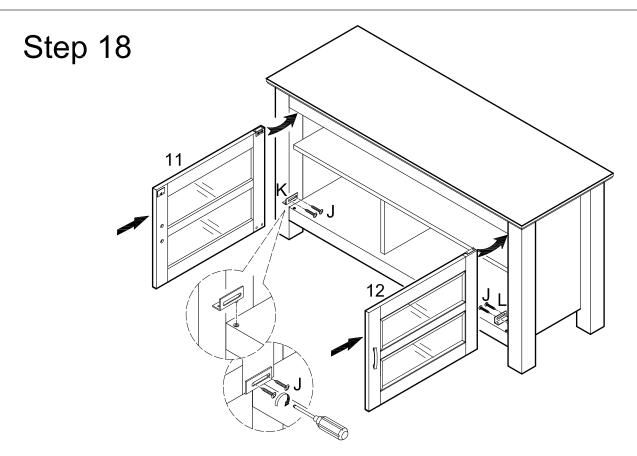
Insert door hinge (K) into left bottom plastic pivot (P). Slide door (11) into place. Attach door hinge (K) to door (11) using screws (J). Insert door hinge (L) into right bottom plastic pivot (P). Slide door (12) into place. Attach door hinge (L) to door (12) using screws (J).
