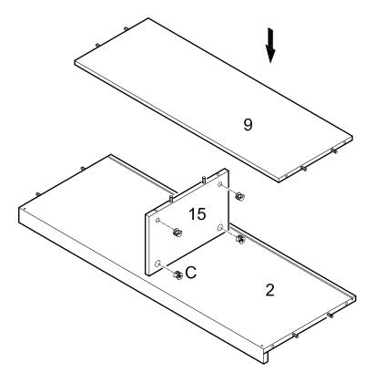
Insert cam locks (C) into panel (15). Attach shelf (9) to panel (15) using cam bolts and dowels as guides. Tighten cam locks (C) with a screwdriver.
