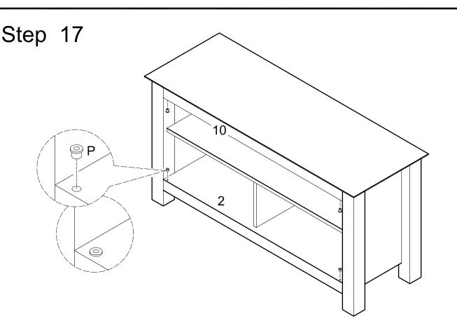
Insert plastic pivots (P) into panel (2) and slat (10).
