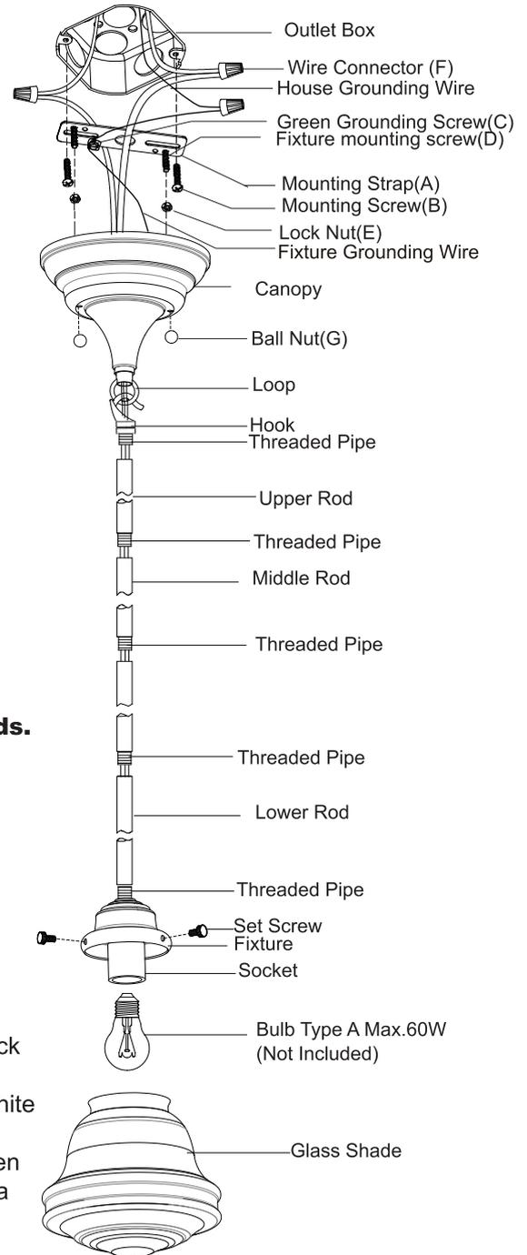
The following parts are available for re-order if damaged or missing.
