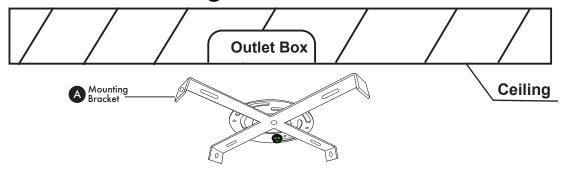
Align mounting bracket (A) with outlet box.
