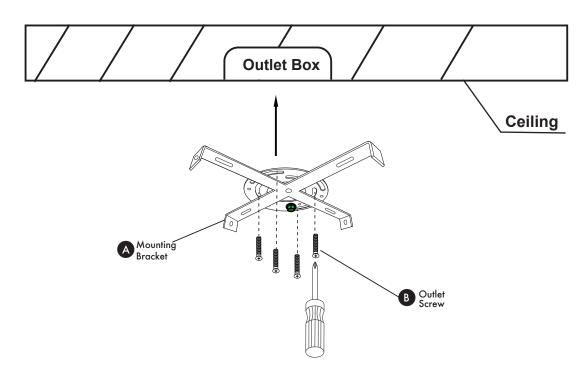
Attach mounting bracket (A) to outlet box. Secure with outlet screws (B).
