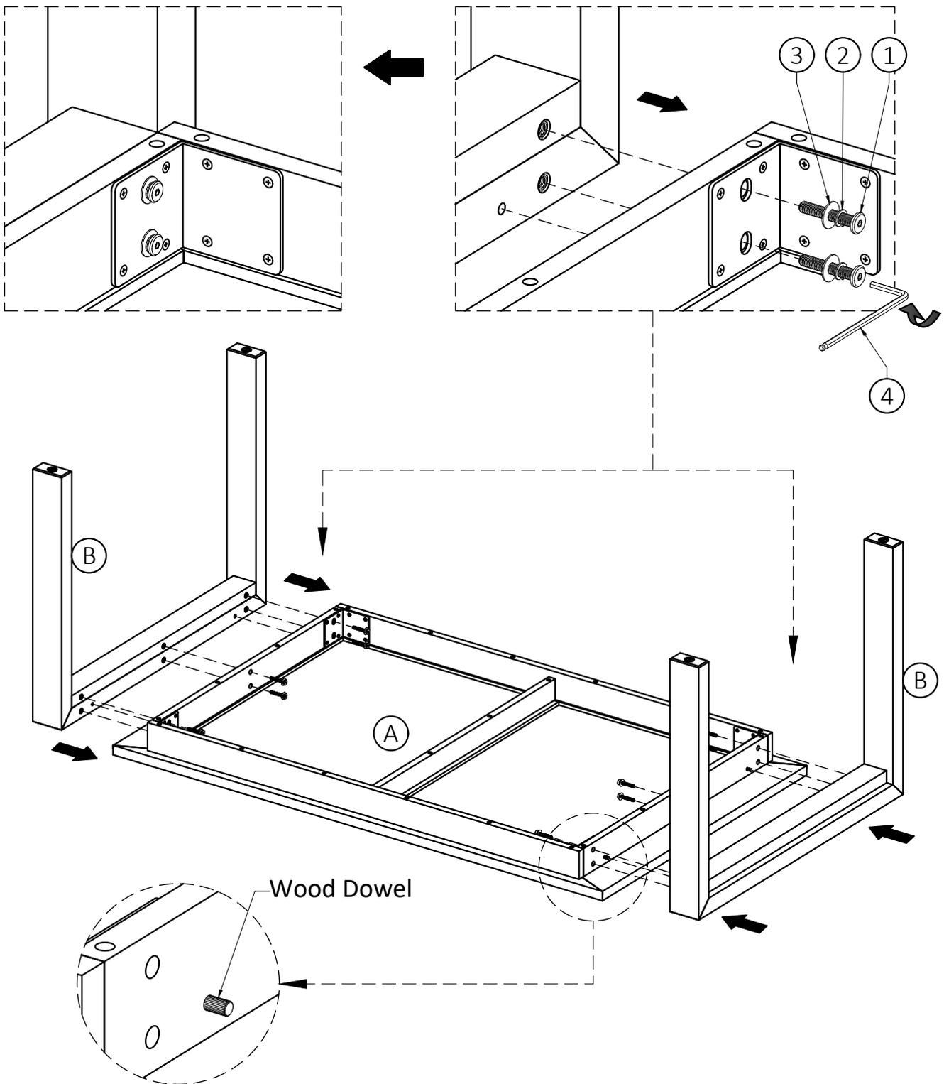
1. Align Wood Dowels with guide holes on Legs (B) and attach Legs (B) to Top (A).
