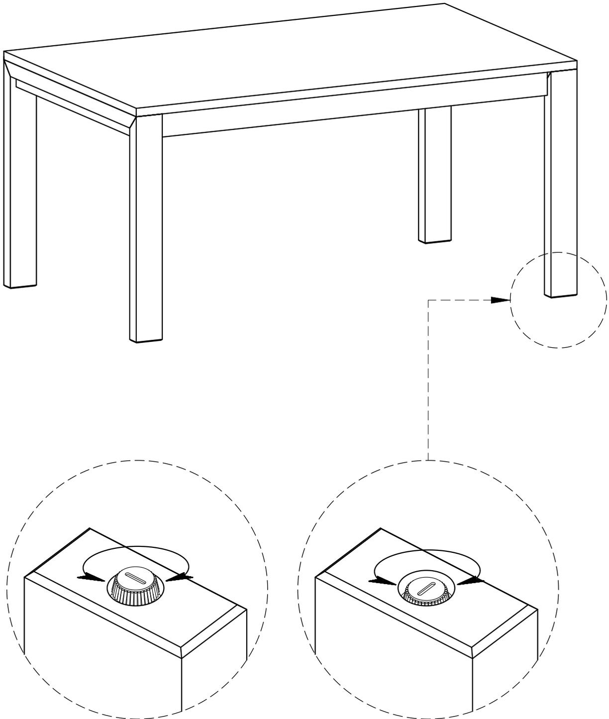
Note: Levelers on bottom of legs can be adjusted if floor is uneven.
