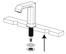
4. Remove the lock nut, metal washer, and rubber waasher from the valve stem labeled 'cold.' Insert the stem into the faucet hole on the right.
