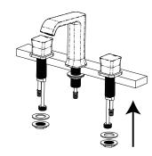
6. Repeat steps 4 and 5 for installing the 'hot' valve stem into the left faucet hole.
