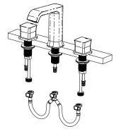
8. Attach the valve stems to the main water supply. Use an adjustable wrench to tighten, but be careful not to overtighten. Apply thread sealant or plumber's tape to each threaded connection. Ensure that you are connecting the hot and cold lines accordingly.
