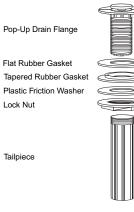
2. Apply plumber's tape to the threading on the tailpiece, then reattach the tail piece to the pop-up drain flange.
