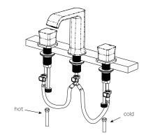
9. Once installation is complete, turn the main water supply back on. Check for any leaks underneath.
