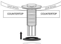
6. Thread the lock nut onto the drain flange. Hand tighten until secure, then finish tightening with a basin wrench once the drain is properly aligned.
