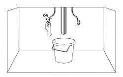
10. Proceed to sink drain installation. Once the drain is installed, turn the faucet on for approximately 60 seconds. Check for any leaks. Test both hot and cold water to ensure they are running properly.
