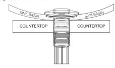
5. From under your counter, slide the tapered rubber gasket followed by the plastic friction washer onto the tailpiece until they meet your sink or countertop. Be sure that the tapered side of the rubber washer is facing up.
